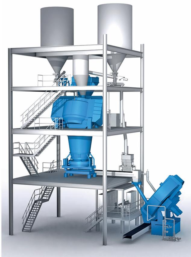
**Figure 6.** The right system concept is key to economic success. Plant design example with mixer and disk pelletiser.
