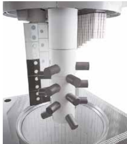
MM3 – Wear elements made of tungsten carbide bar agitator
