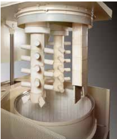
MM5 – Wear elements made of ceramic bar agitator
