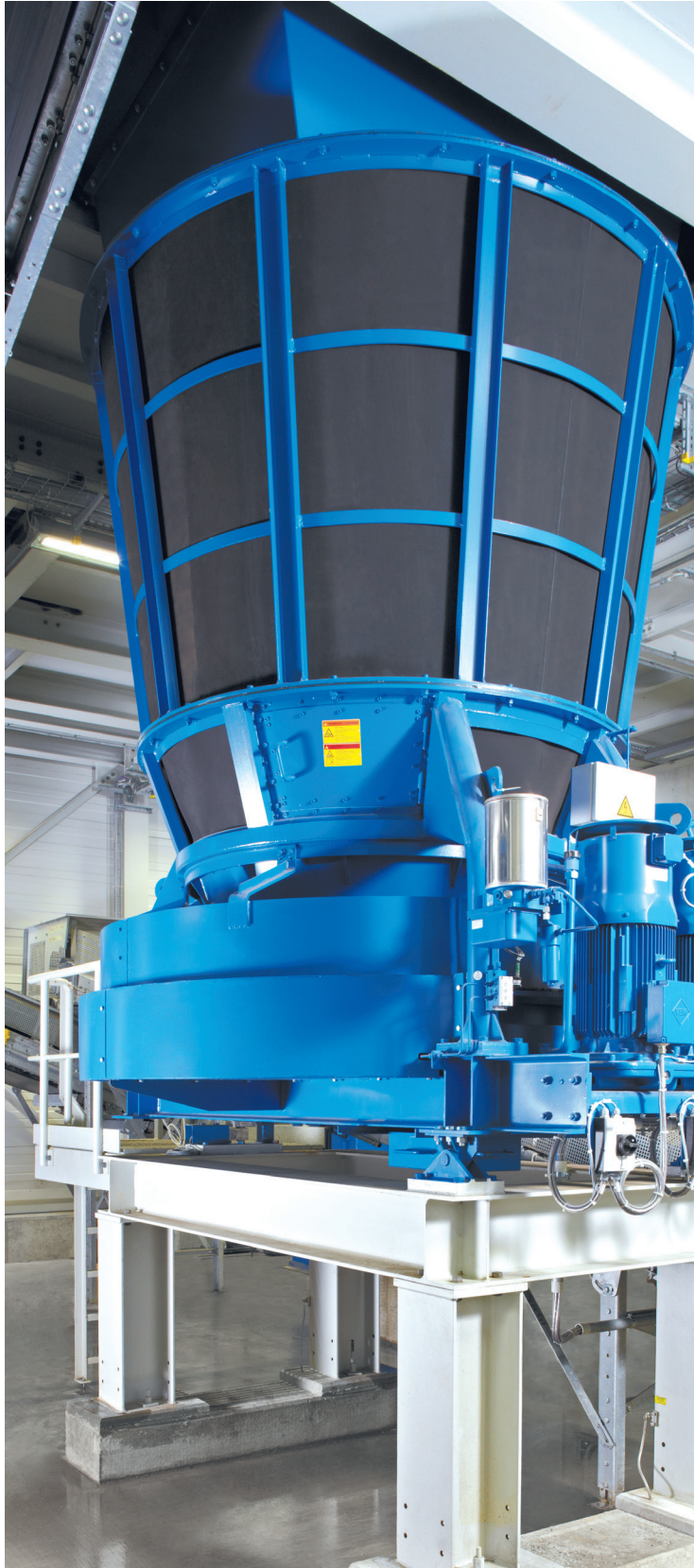
UE25 table feeder in a foundry with a material feed hopper for a volume of 9000 liters
